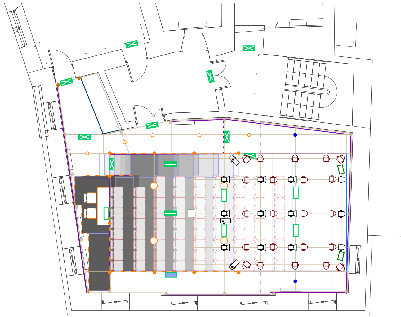
Additional units in crossover under control position and under seating deck
